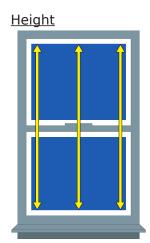
The width and height measurements should be rounded down by a small tolerance of 4mm for fitting the recess in a best possible way.
